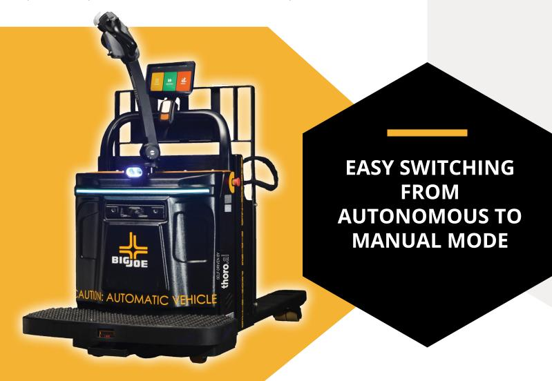
The intuitive software package of the Pallet Mover AMR allows the operator to easily switch the unit from autonomous to manual mode by simply pulling the control handle down into a manual operating position. When an operator has completed their manual operated task, they can resume autonomous mode by allowing the control head to return to its vertical position.
