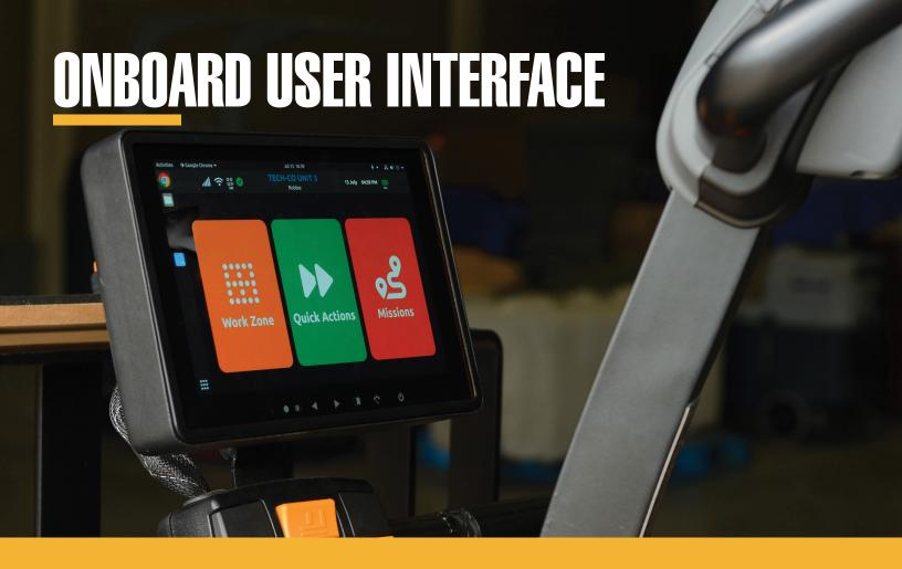
The Pallet Mover AMR features an easy to learn user interface accessed via the onboard touchscreen, allowing you to set-up, map and start missions in less than one hour. If you can use a smartphone, you can program the Pallet Mover AMR!
