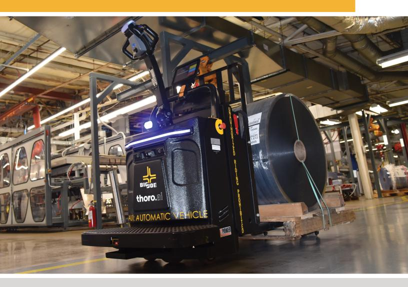
Developed in partnership with Thoro.ai, the Big Joe Pallet Mover AMR is an easy to deploy solution for autonomous floor-to-floor pallet transportation and drop-off that companies can set up and put into operation in less than 1 hour. This new Big Joe unit seeks to revolutionize on-demand material handling across a broad number of industries by offering self-driving technology at an accessible price point on one of the most common material handling vehicles, an electric pallet truck.
