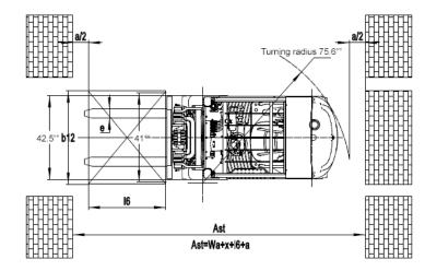
LXE50 Spartan Rated Capacity 5,000lbs. to 130" @ 24" LC 4,000lbs. to 189"/197" @ 24" LC
