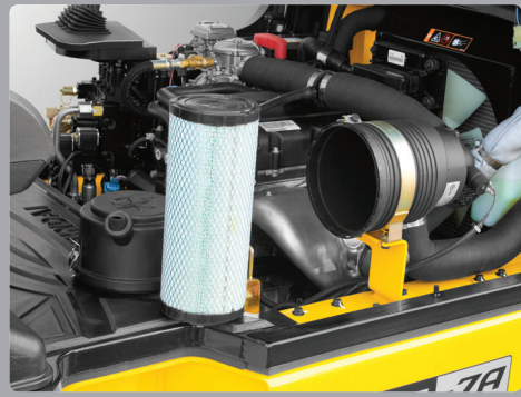
Easy Change Air Cleaner The air filter is readily accessible for cleaning or replacement. (6inch Cyclone Type)
