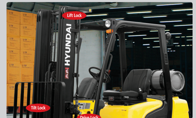
OPSS (Operator Presence Sensing System) Control of mast tilting, lifting and lowering is not possible through operation of the appropriate control when the operator is not in the seated position
